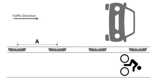
The parallel positioning of TreeTop Premium Rubber Bike Lane Delineators is most suitable when there's limited available buffer zones (i.e.; painted lines). To ensure optimal safety, it is recommended to maintain a spacing between centers (A) of 6ft between the delineators, while not exceeding 8ft.
