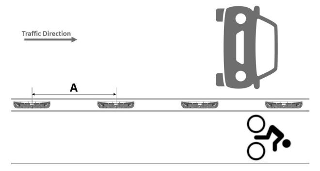
The 5" High Curb Premium Rubber Bike Lane Delineator is designed to deter vehicles from crossing into the bike lane. For applications that require vehicles crossing over, check out Treetop's 3" High Crossover Premium Rubber Bike Lane Delineators.
