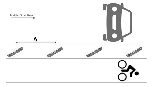
The oblique positioning is recommended when you need to create a wider buffer space for enhanced safety in the bike lane. A wider buffer zones (i.e.; painted lines) contributes to greater safety for cyclists. To ensure optimal safety, it is recommended to maintain a spacing between centers (A) of 6ft between the delineators, while not exceeding 8ft.
