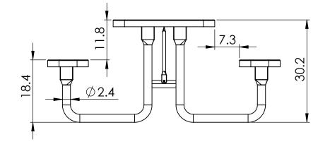
**CONSTRUCTION MATERIAL:** Dia. 2-3/8" #10 GAUGE STEEL TUBULAR FRAME ECOATED AND POWDER-COATED FRAME THERMOPLASTIC COATED STEEL TOPS
