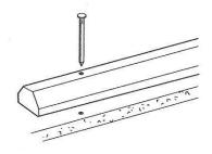
Position parking block in its installation position. Using its pre-drilled holes as a template, mark the location of each hole on the parking surface.
