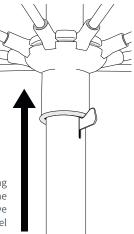
To close your umbrella, begin cranking clockwise until the runner passes the length of the EZ-Up Spring. Once you have cleared the length of the spring, the steel ledge will retract inside of the pole as the you begin to crank counter-clockwise.
