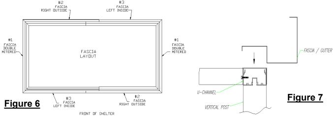
Place a double mitered fascia #1 on a short side of the shelter. The mitered ends of this piece will be visible when looking up at the bottom of the fascia. Repeat process on the other short side of the shelter. **See Figure 7**.
