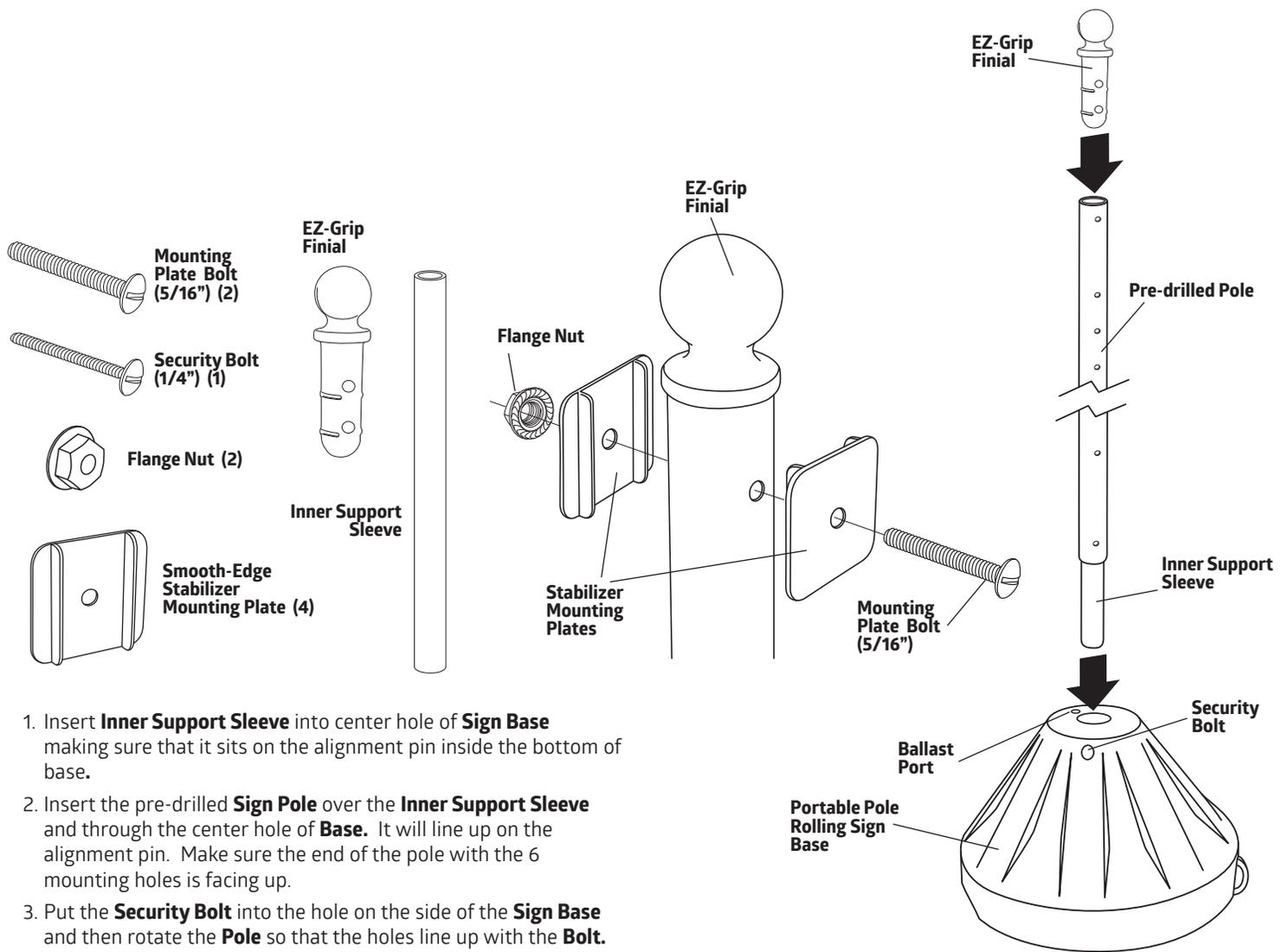
1. Insert **Inner Support Sleeve** into center hole of **Sign Base** making sure that it sits on the alignment pin inside the bottom of base.
