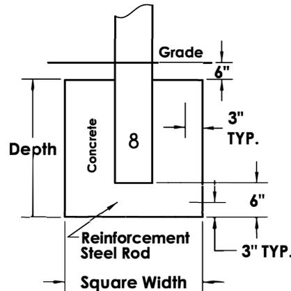
NOTE: A HOLE IS PROVIDED AT THE BASE OF EACH COLUMN FOR ONE #4 ROD
