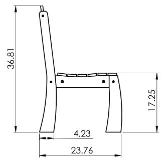
CONSTRUCTION MATERIALS: Recycled Plastic HARDWARE: Stainless Steel
