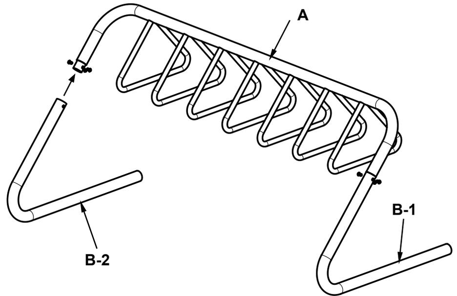
Step 1: According to diagram, attach two ends B-1 and B-2 to A.
