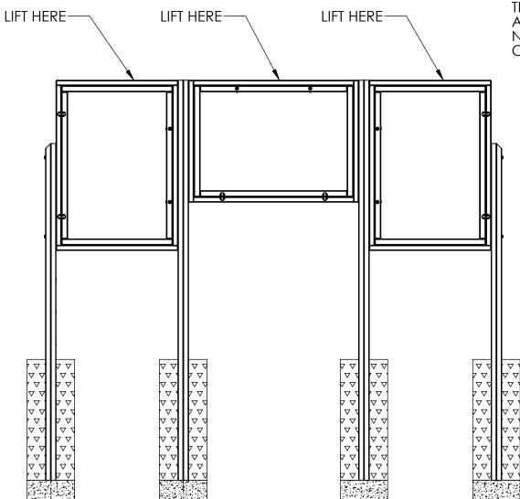
WITH HELP FRONT OTHER PEOPLE, CAREFULLY TILT MESSAGE CENTER ASSEMBLY INTO HOLES AND BRACE MESSAGE CENTER. LEVEL AS NECESSARY AND FILL HOLES WITH READ-TO-MIX CONCRETE. ALLOW TO DRY AND REMOVE BRACING.
