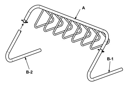
Step 1: According to diagram, attach two ends B-1 and B-2 to A.
