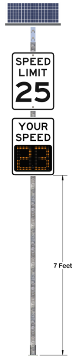
Figure 5-1. Typical DFB Mounting
