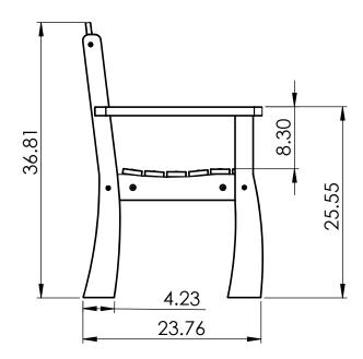
CONSTRUCTION MATERIALS: Recycled Plastic HARDWARE: Stainless Steel
