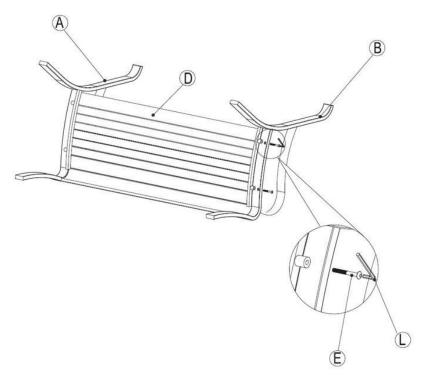
Step # 2: Attach the Backrest (C) to the Left Armrest (B) and Right Armrest (A) by using Short Bolts (F) and Washers (G). Hand tighten! Adjust the bench to a level position and tighten all the Bolts with Allen Wrench (H).
